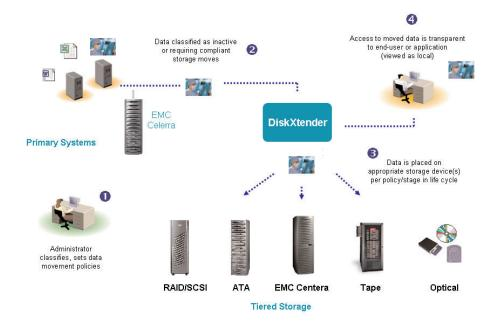
EMC DiskXtender for NAS automatically migrates inactive files from NAS systems to secondary storage devices based on administrator-defined policies. Data movement is transparent to end users.
